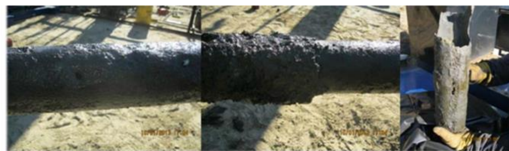
Ref: Corroded production casing pipe sample from downhole (University of North Dakota Energy & Environmental Research Center)
