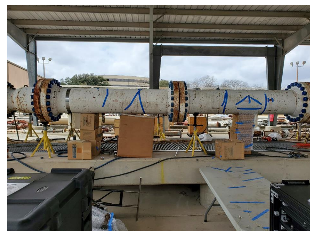
Pilot-scale Demonstration of NETL Optical Fiber Sensors
