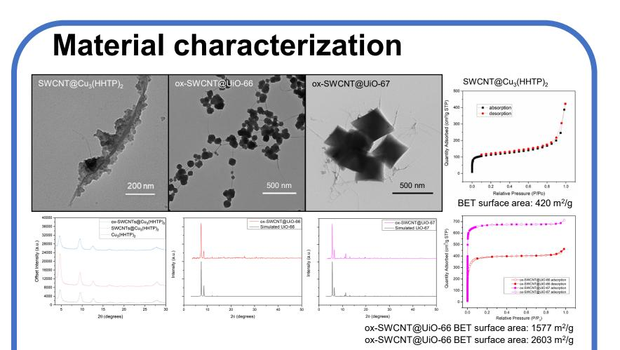
SWCNT@MOF composites combined the porosity of MOF and the electric conductivity of SWCNT. Templated MOF growth was facilitated via  $\pi$ - $\pi$  stacking between the sp<sup>2</sup> carbon of CNT and the MOF ligand and/or the covalent interaction between the carboxylic functionality on oxidized SWCNT (ox-SWCNT) and the MOF metal precursor. MOF chemistry was preserved after hybridization with SWCNT as depicted by the X-ray diffraction (XRD) and  $N_2$  adsorption/desorption isotherm.
