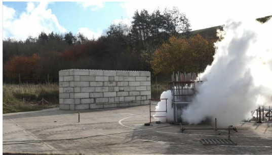
ICHS 183: Visualization and Quantification of Wind-Induced Variability in H2 Clouds Following Releases of Liquid Hydrogen, (I. Palin et al.)
