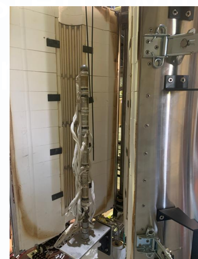
Test of fiber-based H 2 sensor in a solid oxide fuel cell (SOFC). Bottom Left: Inside of SOFC in which the fiber sensor is inserted; Bottom Right: Raman DTS system and SOFC; Top Right: Temperature curves measured via the Raman DTS.
