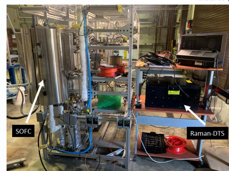
Test of fiber-based H 2 sensor in a solid oxide fuel cell (SOFC). Bottom Left: Inside of SOFC in which the fiber sensor is inserted; Bottom Right: Raman DTS system and SOFC; Top Right: Temperature curves measured via the Raman DTS.
