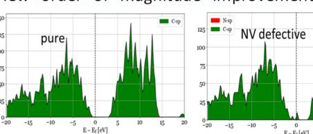
There is a shifting of band edge and splitting of band gap  $\Delta E_{ex}(eV)$ under changes in the lattice parameters (up to  $\pm 2\%$ ).
